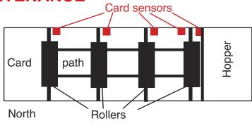
The counters are numbered in the same way as the cards move from the hopper to the left, i.e. in the cards' direction.
